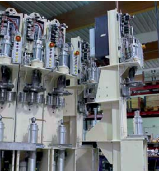
The first modular glass-blowing machine in the world with 24 identically designed, networked stations by Kutzscher, SPS GmbH, and Faschang Werkzeugbau
